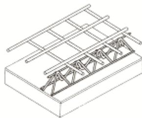
**Linchairs** - Dual Purpose supports for spacing bars and fabric in two metre standard lengths.
