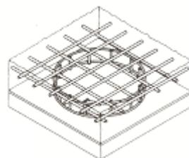
**Circular Spacers** - The most economical way of supporting top steel in slabs with a 3.2/3.6m strip bent and tied to form a 1.000/1.100 diameter circle 2-3 per sheet are normally sufficient.
